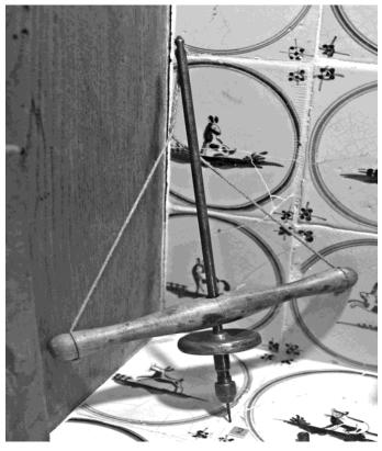
diameter of the hole which is slightly wider than the original diameter of the needle. It is likely that the old oboe makers used similar drills.
