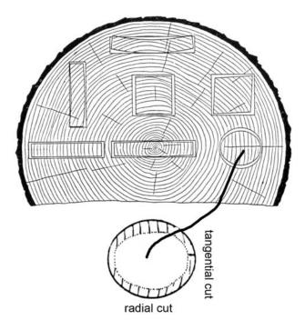
Three of the four boxwood oboes by Hendrik Richters have - as on most Dutch baroque woodwind instruments - the radial cut (or radial face) at the front of the joints. On HR24 this is less clear; the fingerholes about between radial and tangential.
