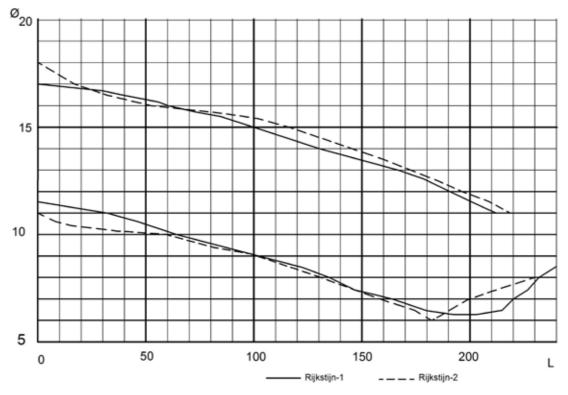
Fig. 13: bore profiles of two oboes by Rijkstijn
