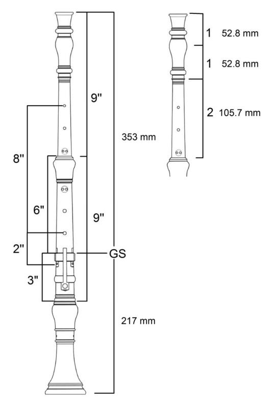
For the design in relation to the proportions of this oboe we must know the length of the sections. At first I look at the oboe with all parts mounted (the tenons are not visible). The lengths of the upper and middle joint are almost the same (211.5 and 212 mm), the bell measures 146.5 mm. We find similar lengths on other Richters oboes.
