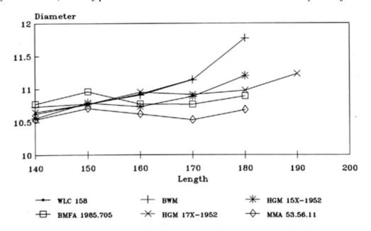
Figure 6: from Adkins 1990: FIGURE 56. Tenon Compression in the Lower 50 mm of the Richters Top-Joint Bores.
