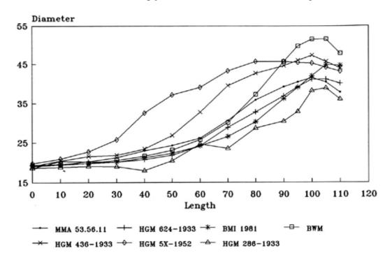
*Fig.* 8: bell bore profiles (from Adkins 1990, fig. 66). MMA = HR16; HGM 624 = FR2; BMI = HR12; BWM = RS5; HGM 436 = HR2; HGM 5-x = RS3; HGM 286 = HR1.
