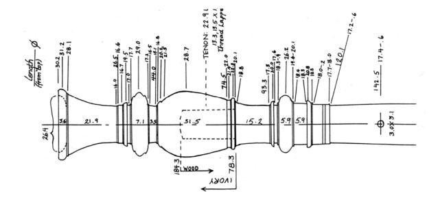
Measurements of the baluster of the oboe 2037 by Hendrik Richters (Bate Collection, Oxford, drawing by Dick Earle, 1989)
