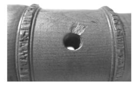
The waist of the bell with resonance holes and 'nibble damage' at the beads.
