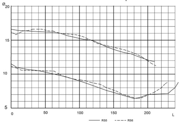
Fig 12: bore profiles of RS5 and RS6
