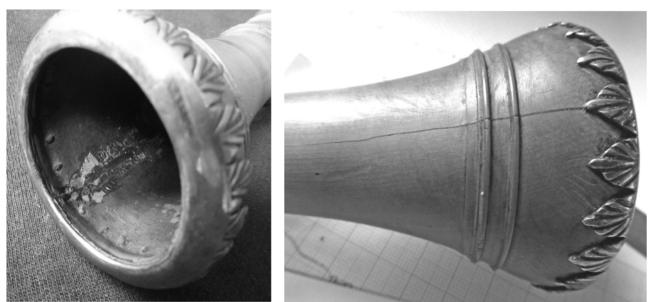
Crack in the wall of the bell
