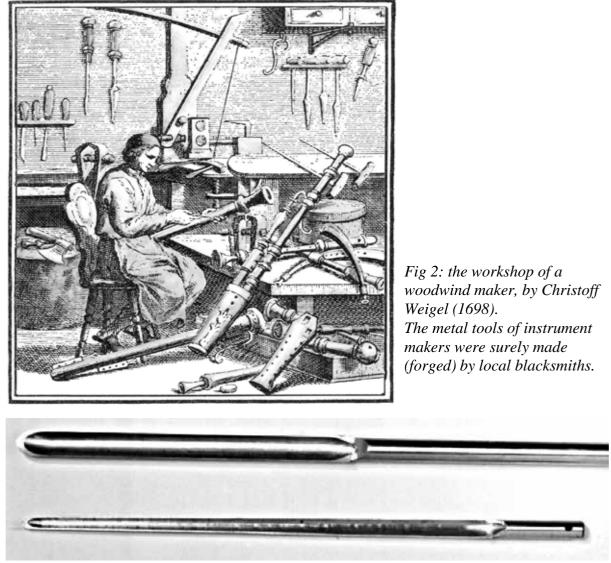
*Figure 3: modern reamers for woodwind instruments, from the website of the firm of Joseph Böhm (Germany). These reamers are made on a modern computerized metal lathe.*
